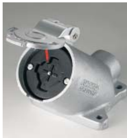
The automatic, positive engagement, single-post design of our Power-Lock® series allows electrical contact to be made only after the locking action is complete, eliminating the risk of air-gap sparking in potentially hazardous environments.
